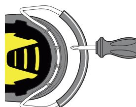
Remove the padding inside the helmet before placing the hat inside.
